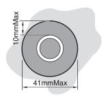
Before installation, installer must provide G1/2" nipple(1). The nipple should extend 11mm beyond the finished wall. Ensure the gap between the nipple and finished wall is no more than 10mm. The hole's maximum diameter is 41mm in the wall.
