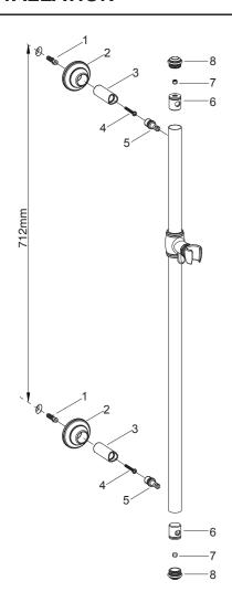
Select a suitable location to drill two holes on the finished wall according to the rough-in dimensions and diameter of the anchor(1), their distance is 712mm. Press the anchors into the holes.
