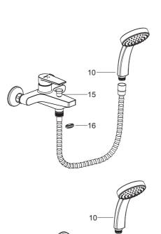
Ensure that all coupling nuts tightened.
