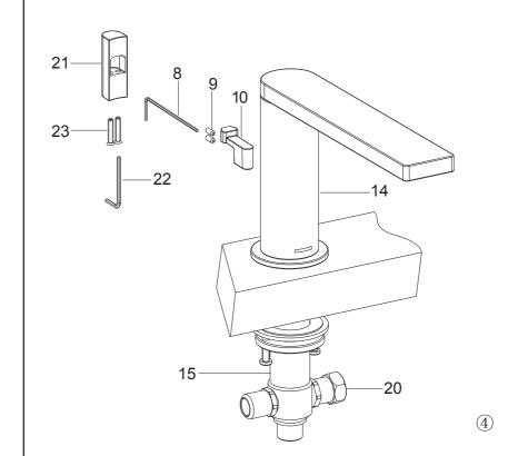
Install the connector(10) to the diverter kit.
