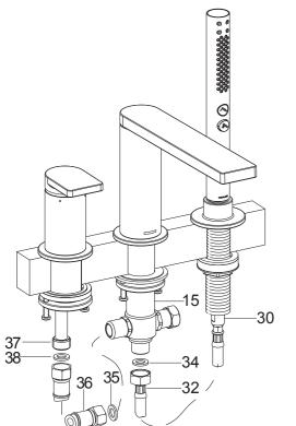
Put the washer(34) into the nut of the hose(32). Connect the connection hose to the diverter kit(15).
