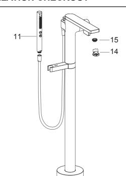
Ensure that all coupling nuts are tight. Ensure that the handle is in the off position.
