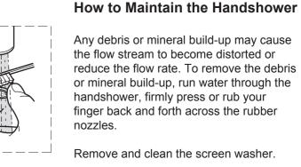
Any debris or mineral build-up may cause the flow stream to become distorted or reduce the flow rate. To remove the debris or mineral build-up, run water through the handshower, firmly press or rub your finger back and forth across the rubber
