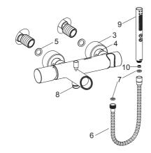
Install the restrictor(10) into the handshower(9) inlet if needed.Connect hose(6) to the faucet outlet(8), and to the handshower with washers(7).
