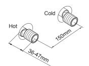
Adjust the center-to-center distance between the connectors to 150mm and horizontal. They should extend 36 to 47mm beyond the finished wall.
