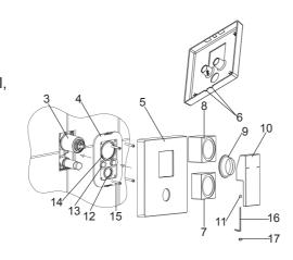
Install handle(10): Tighten the setscrew(11) with hex wrench(16). Press plug button(17) into the hole.
