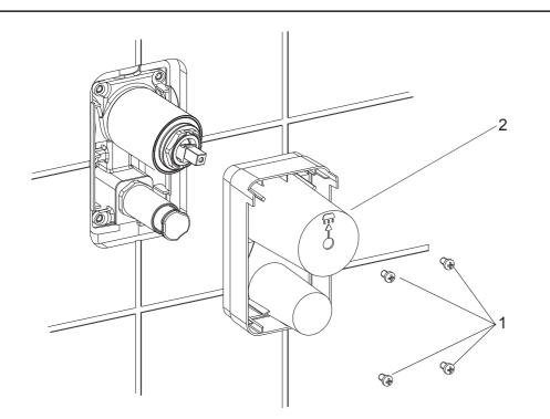
**NOTE:** Install valve 882\* according to the rough-in dimensions of 76966T-4, Install valve 880\* according to the rough-in dimensions of 76967T-4.
