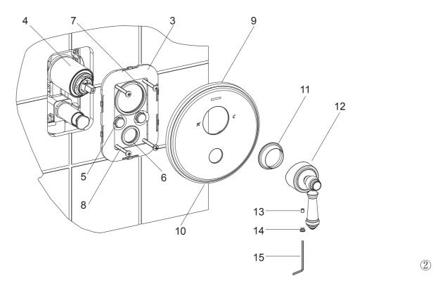
Slide the cover kit(3) onto the valve(4) with the plugs(5) facing outside. **NOTE**: Don't squeeze out the rings(6,7). Push it against the wall.
