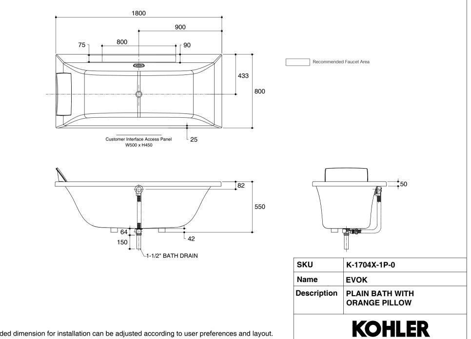
\*The recommended dimension for installation can be adjusted according to user preferences and layout.
