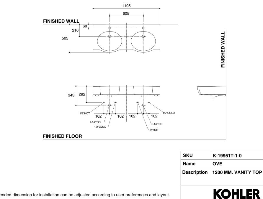
\*The recommended dimension for installation can be adjusted according to user preferences and layout.
