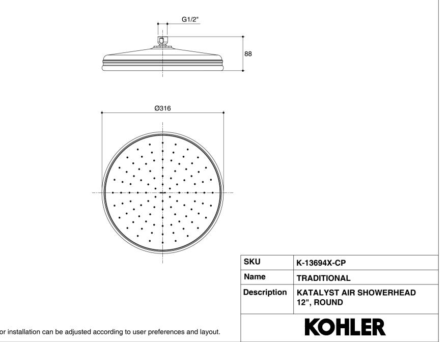
\*The recommended dimension for installation can be adjusted according to user preferences and layout.
