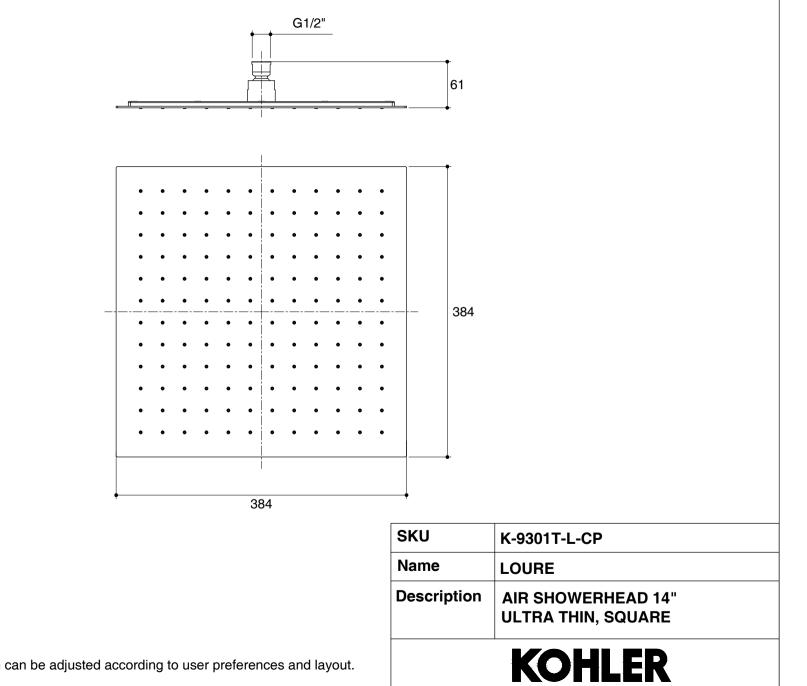
\*The recommended dimension for installation can be adjusted according to user preferences and layout.
