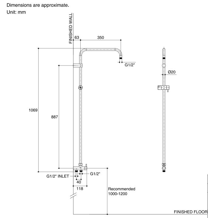
\*The recommended dimension for installation can be adjusted according to user preferences and layout.
